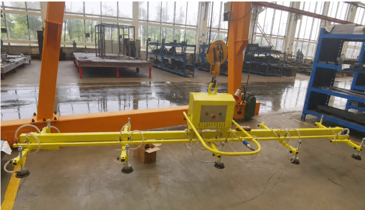
Gantry Crane Steel Plate Handling
