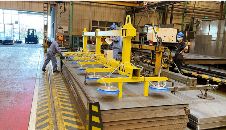
Heavy Steel Plate Handling
