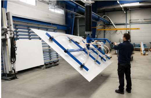
Large Sheet Handling Adjustable multi-cup beams for wide panels and sheet stock.
