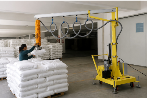
Portable Jib Crane Mobile handling for warehouses, food and chemical processing.
