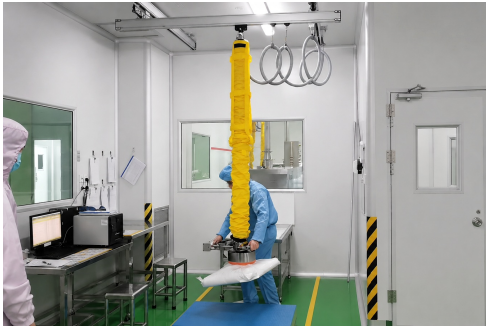
Food-Grade Tube Lifter Bag handling in clean production areas
